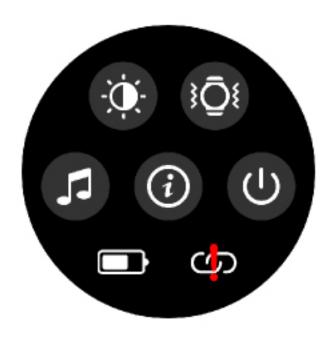
There is a Red line in the Bottom right, which means that the watch's bluetooth is not connected and occupied.
